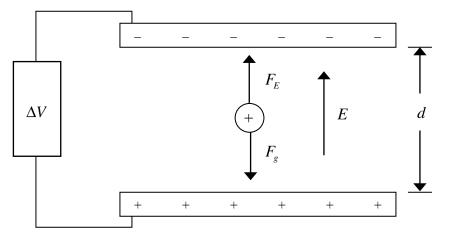
For a positively charged drop of mass m and charge q, the electric force acts upward.
